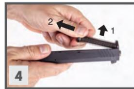
4. Release the **recoil spring assembly** from its position on the bottom of the **barrel**.
