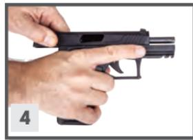
4. Hold the pistol with one hand keeping your finger away from the **trigger**. With the other hand pull the **slide** to its limit and release it, so the **slide** will go forward under **recoil spring** pressure and will insert one cartridge into the **chamber**.
