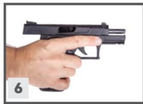
5. The pistol is now ready-to-fire by pulling the **trigger**. After firing, the **slide** will recoil from gas pressure, ejecting the empty case and feed another cartridge into the **chamber** from the **magazine**. The pistol is now ready to fire again.
