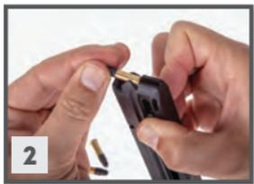
2. To load a **magazine** hold the bottom of the **magazine** with one hand and pull down on the **magazine loading button** using your thumb. With your other thumb insert the cartridges one at a time, pressing them down and to the rear fully under the lips of the **magazine**. Repeat until the **magazine** is loaded to magazine capacity.
